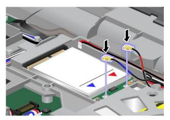
**Note:** Depending on the model, the marking for the connectors on your card might look different from the one shown in the illustration above. Be sure to attach the red cable to the **MAIN** or **M** connector, and the blue cable to the **AUX** or **A** connector.
